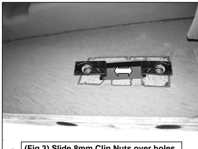
(Fig 3) Slide 8mm Clip Nuts over holes
