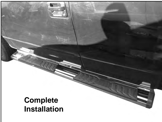
(Fig 11) Driver/left front complete installation
