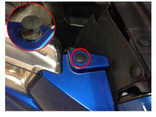
**Step 1:** Using a panel removal tool, remove the push clip holding the headlight cover in place.
