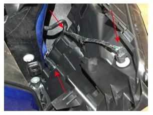
**Step 11:** Remove the (3) headlight bulb connectors, then carefully remove the headlight.
