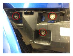
**Step 6:** Remove the (3) 10mm bolts on the side of the headlight nose panel.
