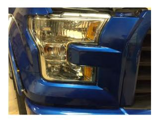
**Step 4:** Carefully pry the headlight bezel away from the headlight. This headlight bezel is held in with clips.
