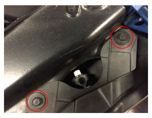
**Step 7:** Remove the (2) 10mm headlight bolts located on the top of the headlight.
