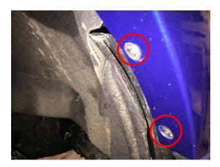
**Step 2:** Using a 7mm socket and ratchet, remove the (2) inner fender flare screws.
