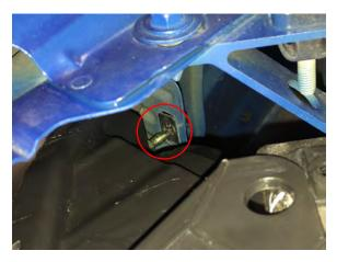
**Step 10:** Carefully pry the headlight away from the locating tab.
