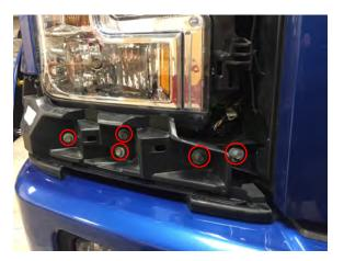
**Step 5:** Remove the (2) 8mm and (3) 10mm bolts on the headlight nose panel.
