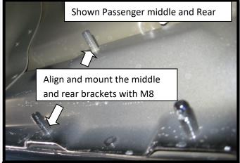
**2.**Attach the passenger middle and rear brackets to the mounting place then secure with M8 nuts. **DO NO TIGHTEN AT THIS TIME**
