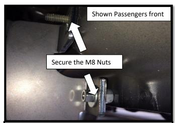
**1.**Attach the passenger front bracket to the mounting place then secure with M8 nuts. **DO NOT TIGHTEN AT THIS TIME**
