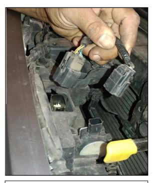
Step 4 Locate and disconnect the 2 electrical plug near the hood latch release.
