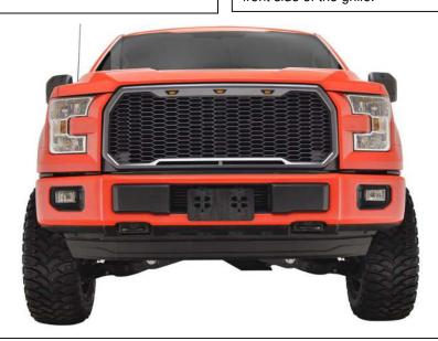
Step 8 Install grille (A) onto vehicle by reversing steps in pages 2-4.
