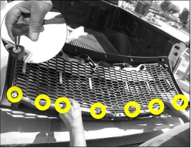
Step 1 Place factory grille bracket onto supplied grille (A). Line up the holes in the factory bracket with the holes in the grille. Step 2
