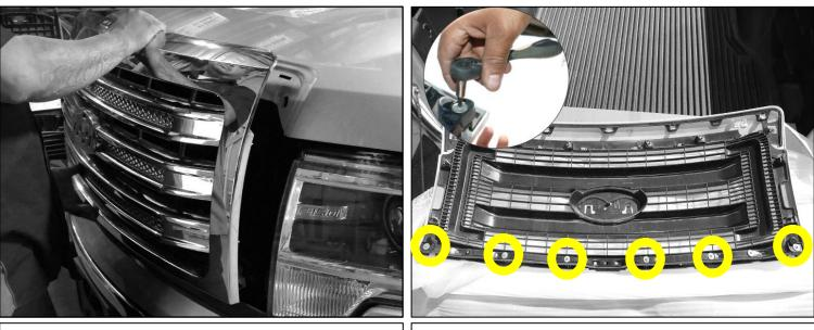
Step 3 Firmly grab and pull factory grille off vehicle. Set factory grille aside in a protected area.
