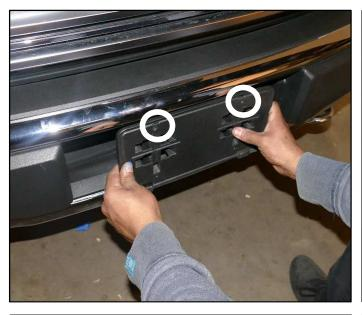
Step 1. Locate and remove two factory screws using a #2 Philips head screwdriver. Firmly grab factory license plate holder and pull away from vehicle. Discard hardware and license plate holder.
