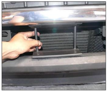
Step 2. Place supplied mounting bracket (B) onto the factory bumper. Line up the holes on the mounting grille with the holes on the factory bumper.
