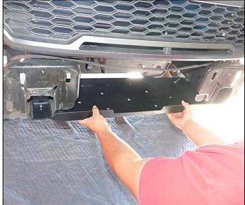
Step 1. Install supplied winch (C) onto vehicle. Line up the holes in the win
