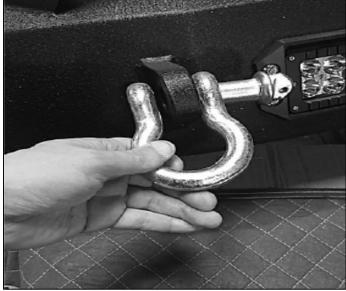
Step 3. Install supplied D-Rings shackles (H) onto D-ring tabs on the bumper.
