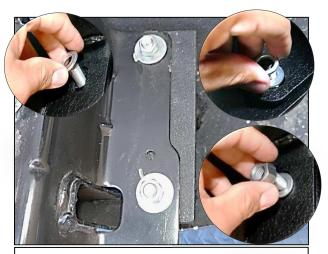
Step 3. Place a supplied M12x1.75 35mm hex head bolt (C) with supplied M12 flat washer (F) from behind the bumper holes and through the holes in the bumper sub frame. Place a supplied M12 flat washer and supplied M12 split washer (E) onto the bolt. Start a supplied M12x1.75 hex head nut onthe bolt. Repeat step for other bolt. Tighten down all hardware using a 18mm wrench. Repeat step for other side.
