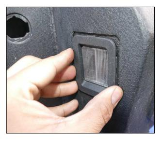
Step 6. Install factory license plate light housing onto new bumper. Repeat for other side.
