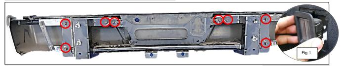
Step 1. Turn factory bumper upside down on work bench. Using a 13mm socket locate and remove 8 factory bolts holding the factory bumper onto the bumper sub frame. Remove factory bumper sub frame from bumper set aside for later use. Discard hardware. At this time remove factory license plate light housing from bumper fig 1 set aside for later use.
