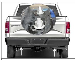
Step 2. Using a 18mm socket locate and remove 4 factory bolts that hold the bumper to the frame of the vehicle (2 on each side). With help from an assistant remove factory bumper from vehicle. Set hardware and bumper aside for later use.
