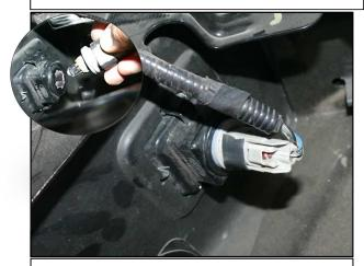
Step 1. Working underneath the vehicle. Disconnect the license plate lights. Repeat for other side. If your vehicle is equipped with a tow hitch receiver plug disconnect at this time.
