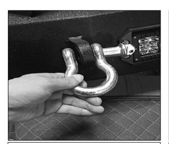
Step 8. Install supplied D-Rings shackles (G) onto D-ring tabs on the bumper.
