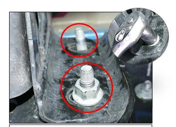
Step 4. With help from an assistant place the supplied bumper (A) onto vehicle as shown above. Line up factory bumper sub frame studs to the vehicle mounting holes. Start factory nuts onto the bolts circled above. Tighten down using 21mm socket. Repeat step for other side.
