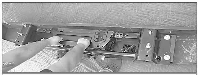
Step 2. Install factory bumper sub frame onto supplied bumper (A) as shown above. Line up bumper sub frame holes with L brackets holes.
