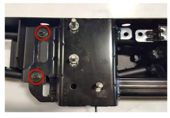
**STEP 8** // If your vehicle is equipped with a factory trailer hitch receiver, remove the (10) factory M10 bolts from the factory bumper. Install the hitch receiver to the Deegan 38 bumper using the (2) double bolt plate, (4) M10 lock nuts, and (4) M10 flat washers.
