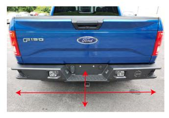
**STEP 11** // Attach the new Deegan 38 bumper to the vehicle using the factory (6) 21mm nuts. Be sure to center the bumper, and adjust height of bumper to desired location.
