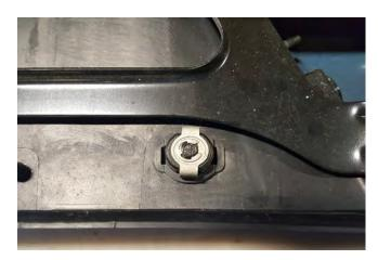
**STEP 4** // Using your factory ignition key, turn the spare tire lock clockwise and remove the spare tire lock from the factory bumper. Then install it in the new Deegan 38 bumper.
