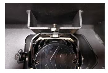
$\begin{tabular}{ll} \textbf{STEP 7} // & \textbf{Install the LED lights using the hardware provided} \\ & \textbf{in the light packaging.} \\ \end{tabular}$
