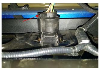
**STEP 1** // Unplug the factory license plate light harness and the trailer plug connector and pull away from the bumper. If equipped unplug and remove the factory backup sensor.
