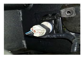
**STEP 12** // Plug the factory license plate lights harness and the trailer plug connector back in. Plug in all factory electrical connections included the license plate lights, trailer plug, and if equipped the reverse sensors.
