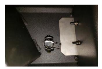
**STEP 10** // If equipped re-install the factory reverse sensors w/ the rubber grommet flush to the outer face of the bumper. \*\*Note: The factory trim bezel does not get re-used. Using the supplied 4mm screws to apply slight pressure to either side of the sensor. Over tightening of the screws can cause sensor damage. For vehicles w/o sensors install the supplied rubber plugs.
