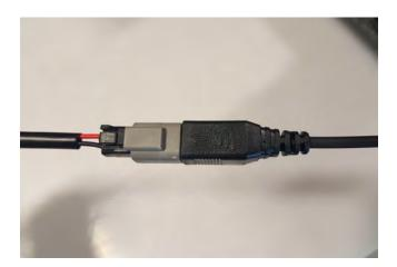
**STEP 13** // Connect the (2) LED fog lights into the supplied harness. Be sure to zip tie the access wiring away from any damage that could occur.
