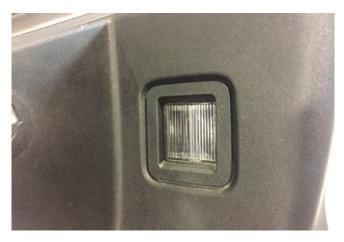
**STEP 5** // Using a flat head screw driver, push in the plastic tabs around the license plate lights, and remove them from the factory bumper. Install these in the new Deegan 38 bumper by pushing them in place till they snap in.
