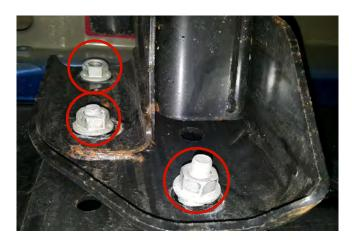
**STEP 2** // Remove the (6) 21mm nuts that hold the bumper to the frame rail. Remove bumper from vehicle.
