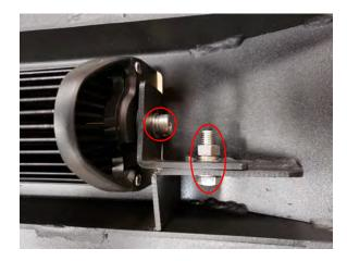
**STEP 10** // Install the (2) LED light bar mounting brackets to the grille using the (2) M8x25mm hex bolts, (4) flat washers, (2) lock washers, and (2) nuts. Then install the (1) 30" light bar to the bracket using the supplied hardware.
