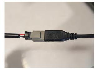
**STEP 14 //** Connect the (1) LED lightbar into the supplied harness. Be sure to zip tie the access wiring away from any damage that could occur.
