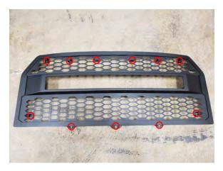
**STEP 11 //** Install the new Deegan 38 grille to the factory base by using the (8) M6x30mm allen bolts, (12) flat washers, (4) lock nuts, and (4) speed clips on the sides and across the top. Then install the (3) M6x25mm allen bolts, (6) flat washers, and (3) lock nuts across the bottom.
