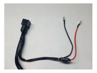
**STEP 15** // Install the Red 12+ volt wire to the positive battery terminal. Connect the Black ground wire ot the negative battery terminal. Mount the fuse in a safe location away from any damage that could occur. Tuck away any extra wiring.
