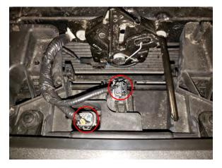
**STEP 4** // Carefully unplug the wiring connections for the grille's shutter system to the factory grille.
