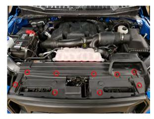
**STEP 1 //** Begin by locating the (9) plastic push clips securing the factory radiator cover, and remove using a trim panel removal tool.
