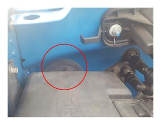
**STEP 16** // Route the on/off switch to the interior of the vehicle using a suitable body grommet. Mount the switch in the desired location. Zip tie any extra loose wiring away from any damage that could occur.
