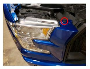
**STEP 2 //** Using a trim panel removal tool, remove the push clip securing the upper headlight bezel in place.
