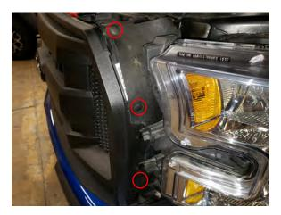
**STEP 6 //** Using a trim panel removal tool, remove the (3) push clips securing the heat shielding to the factory grille.
