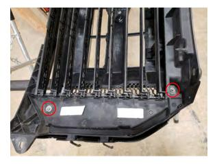
**STEP 9** // Separate the grille from the base by removing the (2) 10mm lock nuts on each side of the grille. Then remove the (3) 10mm nuts across the bottom. The grille will now separate from the base.
