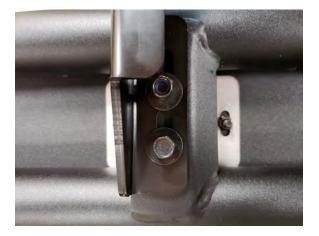
**STEP 4 //** Install the (3) brackets to the side step by using the (3) stud plates, (3) M10 bolts with washers, (3) M10 flat washers, and (3) lock nuts. \*\*Note do not fully tighten.
