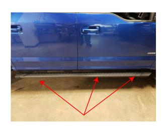
**STEP 1 //** Begin by locating the (3) body mount mounting locations under the vehicle.
