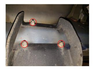
**STEP 2 //** From under the vehicle, remove all (3) 13mm nuts holding the factory side step to each of the body mounts of the vehicle.
