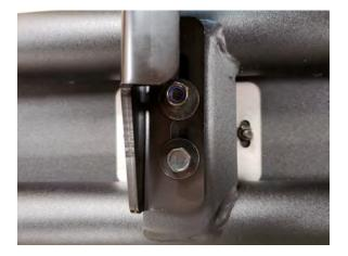
**STEP 4 //** Install the (2) brackets to the side step by using the (2) stud plates, (2) M10 bolts with washers, (2) M10 flat washers, and (2) lock nuts. \*\*Note do not fully tighten.
