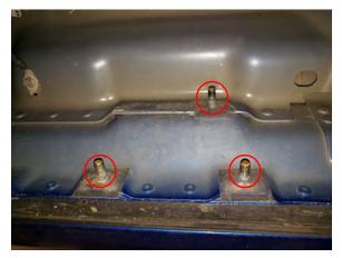
**STEP 3 //** Carefully pull the side step away from the vehicle and downward to remove from the vehicle. Take this time to clean the body mounts, and bolt studs from any road debris.
