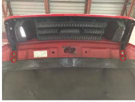
**Step 1//**Begin by raising the hood to access the grille mounting hardware. Remove the (4) 10mm bolts that hold the grille brace to the hood.
