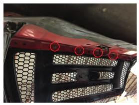
**Step 2//**Then remove the (4) 10mm nuts that secure the grille to the top of the hood. Carefully Remove the grille from the vehicle.
