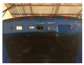
**Step 1//** Begin by opening the hood and removing the (4) factory weatherstripping push pins.
