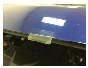
Before installing the Bug Deflector, align the mounting holes and line up the vinyl squares with the metal clips. Place the supplied vinyl squares on the hood surface where the metal clips secure the outer edges of the Bug Deflector. Fold the square around to the backside to protect the paint on the top and bottom of the hood.
