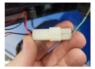
**Step 5**\\ Connect the new Axial mirror light harness to the factory mirror light harness.
