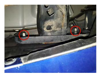
**STEP 2** // From under the vehicle, unplug the factory fog light connectors. Remove the (4) 21mm nuts holding the front bumper to the frame rail of the vehicle. Remove the bumper. \*\*Note: Factory hardware will be reused.
