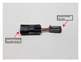
**STEP 14** // Using the supplied (2) fog light adaptor harnesses, connect one end to the vehicles factory fog light harness, and the opposite end to the new Deegan 38 fog light.
