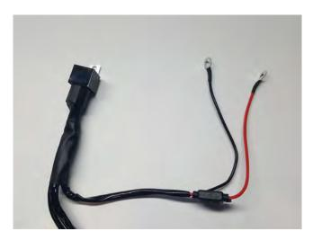
**STEP 16** // **Optional LED Lightbar Wiring:** Install the Red 12+volt wire to the positive battery terminal. Connect the black ground wire to the negative battery terminal. Mount the fuse in a safe location away from any damage that could occur. Tuck away any extra wiring.
