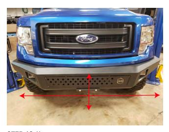
**STEP 12** // Slide bumper into place, and secure using the factory hardware. Be sure to center the bumper, and adjust height of bumper to desired location. Once desired location is met, torque to 40 ft-lbs.
