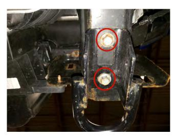
STEP 4 // If vehicle is equipped with the factory tow hooks, remove the (2) 18mm bolts securing the tow hooks to the frame rail. Then reinstall the tow hooks spacing them away from the frame rail using the (2) spacers, (2) M12x55 bolts, flat washers, and lock washers.
