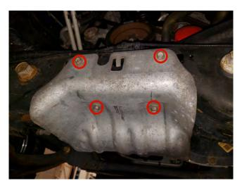
**STEP 3** // From under the vehicle, locate and remove the (4) 15mm bolts securing the factory skid plate in place. Remove skid plate.
