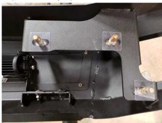
**STEP 7** // Using the supplied (6) plastic bolt holders, attach the factory bolts to the Deegan 38 bumper.
