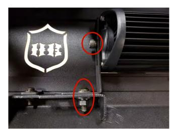
**STEP 6** // If purchased with the LED lightbar option, install the (2) LED light bar brackets, (2) M8x25mm allen bolts, (4) M8 flat washers, (2) M8 lock washers, and (2) M8 nuts to the lower part of the bumper. Install the (1) LED light bar to the upper part of the LED light bar bracket using the (2) M8x20mm allen bolts, and lock washers. \*\*Note: If you did not purchase the LED light bar option, use solid mesh grille option.
