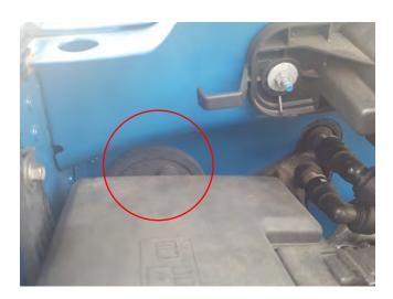
**STEP 17** // **Optional LED Lightbar Wiring:** Route the on/off switch to the interior of the vehicle using a suitable body grommet. Mount the switch in the desired location. Zip tie any extra loose wiring away from any damage that could occur.
