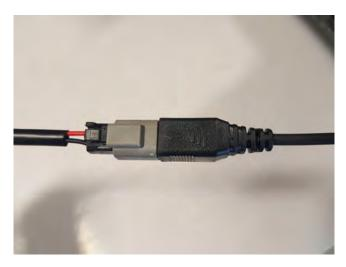
**STEP 15** // Optional LED Lightbar Wiring: Connect the (1) LED Lightbar into the supplied harness. Be sure to zip tie the access wiring away from any damage that could occur.
