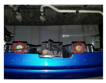
STEP 1 // Remove the (2) 8mm screws that hold the hood latch to the factory bumper.
