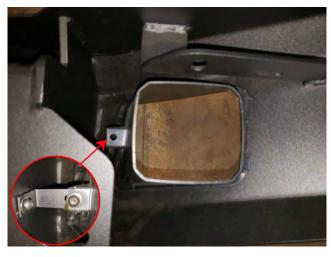
**STEP 8** // Using a 10mm wrench, allen wrench, (2) M8 allen bolts, and (2) M8 nuts, install the fog light bezels to each side of the bumper.
