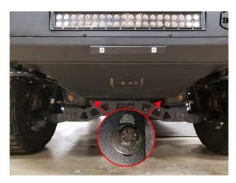
**STEP 13** // Install the rear section of the skid plate to the core support of the vehicle and into the c-clips installed in step 11 using the (2) M12 t-bolts, flat washers, and lock washers.
