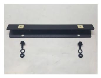
**STEP 5** // Attach the front license plate bracket to the new Deegan 38 bumper if a front license plate is required using the (2) M6 screws, lock washers, and nuts.
