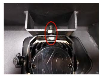
**STEP 9** // Install the LED lights using the hardware provided in the light packaging.
