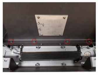
**STEP 10** // Install the Deegan 38 skid plate to the bumper using the (4) M8x25 hex bolts, (8) flat washers, (4) lock washers, and (4) nuts.
