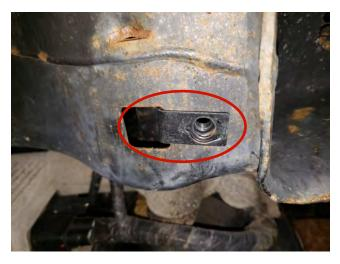
**STEP 11** // From under the vehicle, locate and insert the (2) skid plate c-clips into the factory core support.
