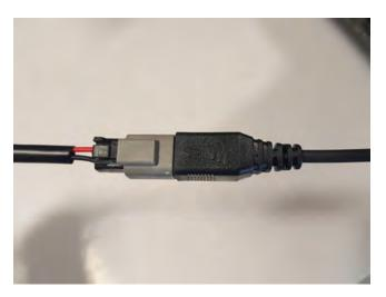
**STEP 10** // Connect the (2) LED Fog lights into the supplied harness. Be sure to zip tie the access wiring away from any damage that could occur.
