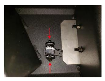
**STEP 7** // If equipped re-install the factory reverse sensors w/ the rubber grommet flush to the outer face of the bumper. \*\*Note: The factory trim bezel does not get re-used. Using the supplied 4mm screws to apply slight pressure to either side of the sensor. Over tightening of the screws can cause sensor damage. For vehicles w/o sensors install the supplied rubber plugs.
