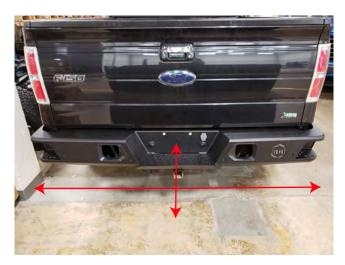
**STEP 9b** // Attach the new Deegan 38 bumper to the vehicle using the factory (6) 21mm nuts. Be sure to center the bumper, and adjust height of bumper to desired location. Then reinstall the trailer plug and license plate harnesses. If equipped, reinstall the backup camera harnesses.
