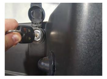
**STEP 3** // Using your factory ignition key, turn the spare tire lock counter clockwise and remove the spare tire lock from the factory bumper. Transfer it to the new Deegan 38 bumper.
