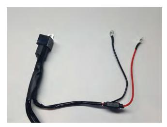
**STEP 11** // Install the Red 12+ volt wire to the positive battery terminal. Connect the Black ground wire to the negative battery terminal. Mount the fuse in a safe location away from any damage that could occur. Tuck away any extra wiring.
