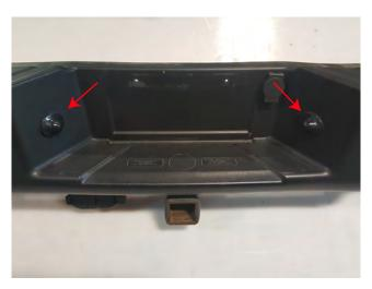
**STEP 4** // Using a trim panel removal tool, push in the plastic tabs around the license plate lights and remove them from the factory bumper. Install these in the new Deegan 38 bumper by gently pushing them in place until they click in.
