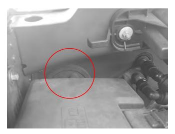
**STEP 12** // Route the on/off switch to the interior of the vehicle using a suitable body grommet. Mount the swtich in the desired location. Zip tie any extra loose wiring away from any damage that could occur. Installation is now complete.
