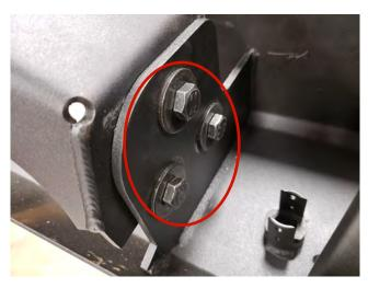
**STEP 8** // If your vehicle is not equipped with a trailer hitch receiver, install the two rear bumper brackets to the bumper using the (3) M12x50 bolts, (6) M12 flat washers, and (3) M12 lock nuts. Then install the factory triple bolt plate through the back of the mounting tabs.
