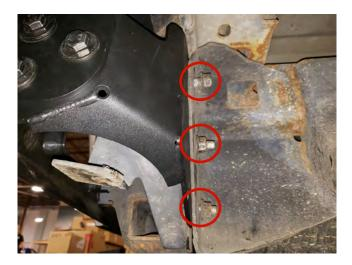
**STEP 9a** // If your vehicle is equipped with a factory trailer hitch receiver, install the two rear bumper brackets to the bumper using the (3) M12x50 bolts, (6) M12 flat washers, and (3) M12 lock nuts. Then remove the (6) factory M8 bolts from the factory bumper, and remove the hitch receiver assembly. Install the hitch receiver through the rear bumper brackets holes.
