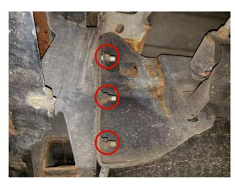
**STEP 2** // From under the vehicle, remove the (6) 21mm nuts holding the rear bumper to the frame rail of the vehicle. Remove the bumper. \*\*Note: Factory hardware will be reused.
