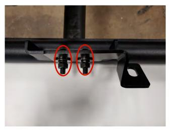
**STEP 5** // Install the (2) inner mid plate brackets with the optional (2) grille lightbar brackets using the (2) M8x30 allen bolts, (4) flat washers, (2) lock washers, and (2) nuts. Repeat on each side.
