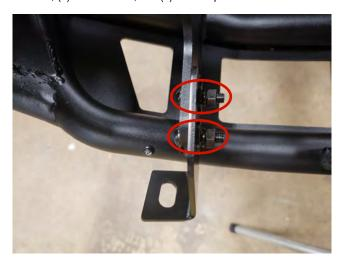
**STEP 6** // Install the (2) inner mid plate brackets using the (2) M8x30 allen bolts, (4) flat washers, (2) lock washers, and (2) nuts. Repeat on each side.
