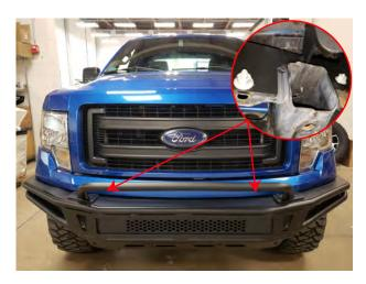
**STEP 10** // Attach the bumper to the vehicle using the factory hardware. Be sure to center the bumper, and adjust height to desired location.
