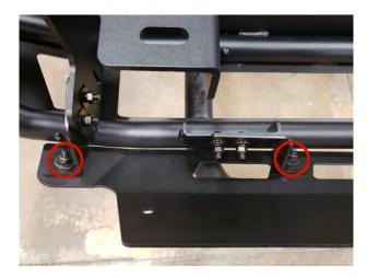
**STEP 7** // Install the mid plate to the bumper using the (2) M8x30 allen bolts, (4) flat washers, (2) lock washers, and (2) nuts. Repeat on each side.
