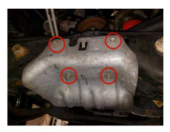
**STEP 9** // Locate, and remove the (4) 15mm bolts securing the factory skid plate. Remove skid plate.
