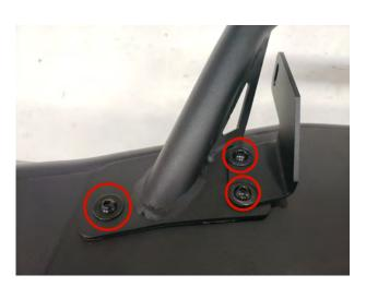
**STEP 4** // Install the optional overrider bar with the optional (2) lightbar mounts onto the bumper using the (3) M8x30 allen bolts, (6) M8 flat washers, (3) M8 lock washers, and (3) M8 nuts. Repeat on opposite side. If choosing to not use the overrider bar, use the (2) overrider block off plates.
