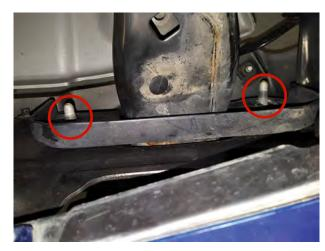
**STEP 2** // Next, loosen the upper (4) 21mm nuts holding the front bumper to the support beam of the vehicle. Remove bumper. \*\*Note: Factory hardware will be reused.
