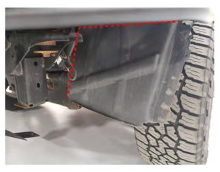
**STEP 12** // Remove / modify / secure the factory inner fender liners. Secure any and all factory components away from tire or suspension components. Installation is now complete.
