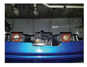
**STEP 1** // Open the hood. Locate and remove the (2) 8mm screws that hold the hood latch release plate to the factory bumper lip.
