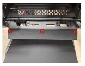
**STEP 8**// Attach the skid plate to the mid plate using (3) M8x30 allen bolts, (6) M8 flat washers, (3) M8 lock washers, and (3) M8 nuts.
