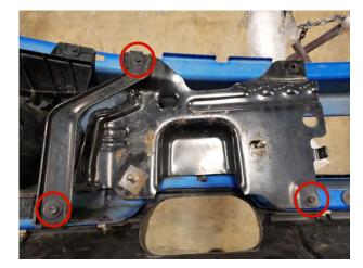
**STEP 3** // Remove the (3) 10mm bolts on each side of the factory bumper, and remove the dual bolt plate. This will be used to secure the new bumper.
