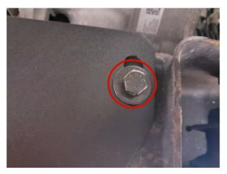
**STEP 11** // Insert the (2) speed clips into the body of the vehicle and secure the skid plate to the vehicle using the (2) M10x30 bolts, flat washers, and lock washers.
