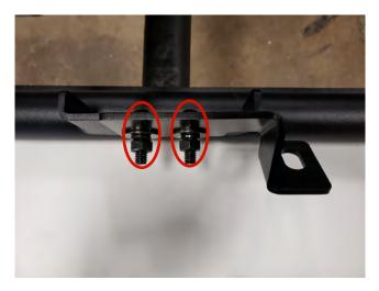
**STEP 5** // Install the (2) inner mid plate brackets with the optional (2) grille lightbar brackets using the (2) M8x30 allen bolts, (4) flat washers, (2) lock washers, and (2) nuts. Repeat on opposite side.
