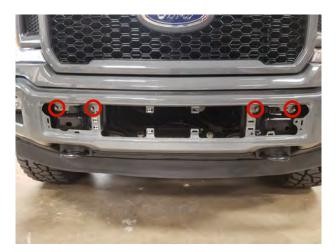
**STEP 2** // Next, loosen the upper (4) 21mm nuts holding the front bumper to the support beam of the vehicle. \*\*Note: Factory hardware will be reused.
