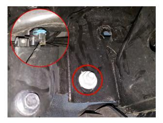
**STEP 3** // Unplug the factory fog light connectors on each side and unclip the wiring harness from the bumper. Remove the lower (2) 21mm nuts, one on each side. Then remove the front bumper from the vehicle. \*\*Note: Factory hardware will be reused.
