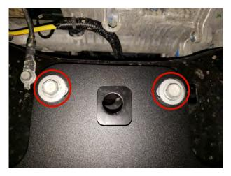
**STEP 11** // Using the factory hardware from Step 9, secure the skid plate to the vehicle to the factory power steering skid plate location.
