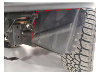
**STEP 12** // Remove / modify / secure the factory inner fender liners. Secure any and all factory components away from tire or suspension components. Installation is now complete.
