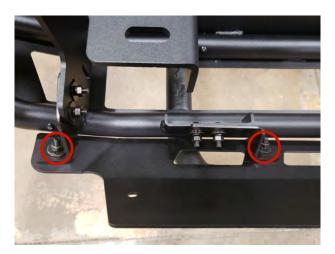
**STEP 7** // Install the mid plate to the bumper using the (2) M8x30 allen bolts, (4) flat washers, (2) lock washers, and (2) nuts. Repeat on opposite side.
