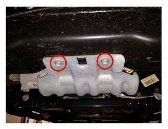
**STEP 9** // Locate, and remove the (2) 15mm bolts securing the factory skid plate covering the power steering.. Remove skid plate. \*\*Note: Factory hardware will be reused.
