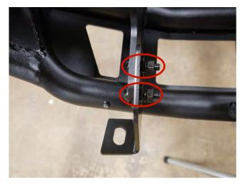
**STEP 6** // Install the (2) inner mid plate brackets using the (2) M8x30 allen bolts, (4) flat washers, (2) lock washers, and (2) nuts. Repeat on opposite side.
