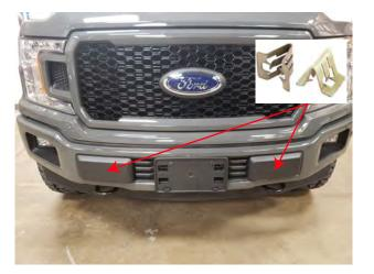
**STEP 1** // Using a panel removal tool, remove the plastic bumper insert. It is held in with several metal push clips.
