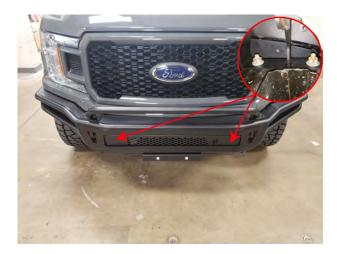
**STEP 10** // Attach the bumper to the vehcile using the factory hardware. Be sure to center the bumper, and adjust height to desired location.
