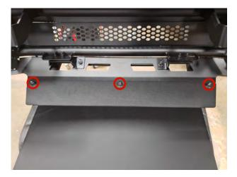
**STEP 8**// Attach the skid plate to the mid plate using (3) M8x30 allen bolts, (6) M8 flat washers, (3) M8 lock washers, and (3) M8 nuts.
