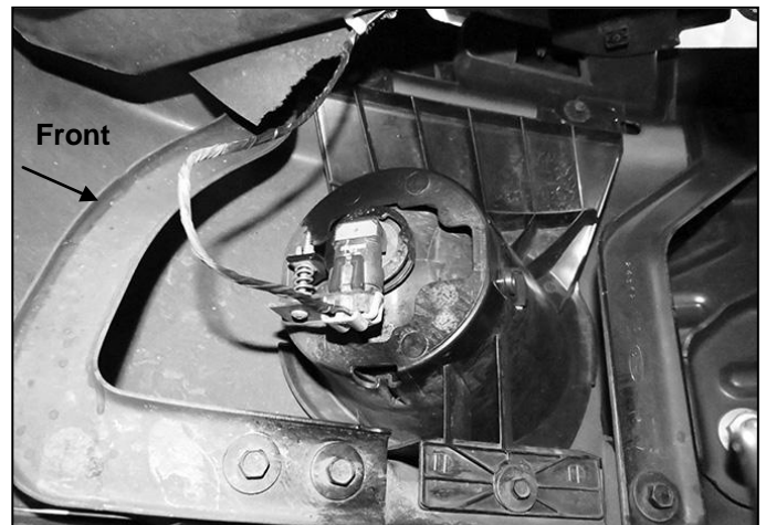
(Fig 2) Unplug factory fog light if equipped. Release clips and move wire harness away from bumper
