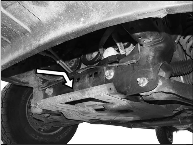
(Fig 1) Example of “flat style” factory skid plate. Insert end of LD-2 Skid Plate between factory skid plate and crossmember (arrow)
