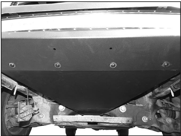
(Fig 8) Skid Plate fully installed on model with “flat style” factory skid plate
