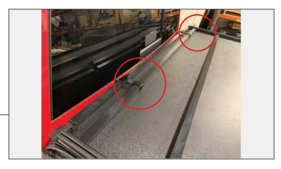
Place the tonneau cover on the bed of the vehicle. The shorter latch component will be closest to the cab. The longer strap component will be on top.
