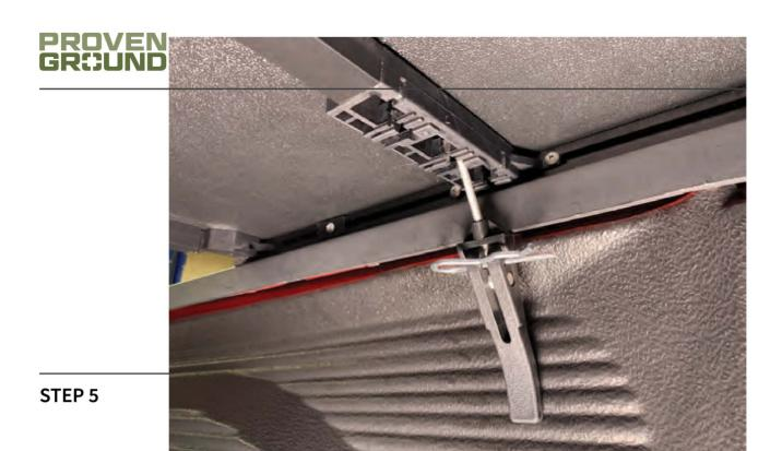
With the latches secured, install the supplied cotter pins to lock them in place.
