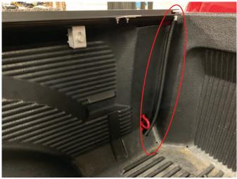
**Step 1\\**Begin my installing the drain tubes on the tonneau cover rails. The drains are located on the cab side of the rails.
