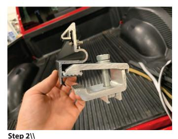
Slide the rail clamps into the bed rails as shown.
