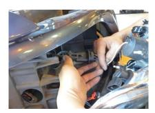
Step 9: Plug in the headlight harness into the new headlight assembly.
