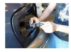
Step 6: Remove corner bulb out from the harness.
