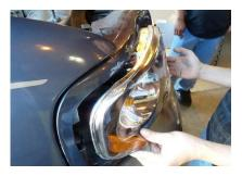
Step 10: Align the headlight and place back into housing.
