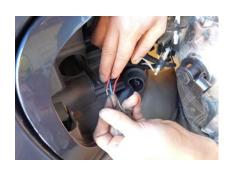
Step 8: Splice the led wires into the corner light. Blue wire (+) will be positive splice into the brown wire on the corner light. Black wire (-) negative will be spliced in to the black wire on the corner light.
