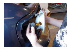
Step 5: Remove the bulb from the corner light.
