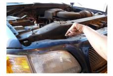
Step 3: Pull off the headlight assembly straight out from the
