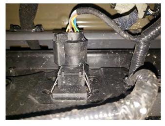
**STEP 1** // Unplug the factory license plate light harnesses, and the trailer plug connector and pull away from the bumper. If equipped unplug and remove the factory backup sensors.
