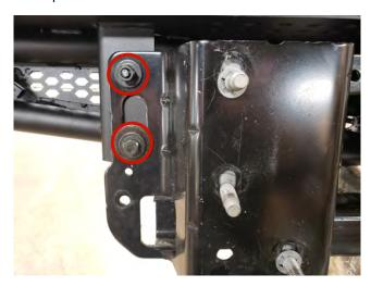
**STEP 8b** // If your vehicle is equipped with a factory trailer hitch receiver, remove the (3) factory 10mm bolts on each side from the factory bumper, and remove the hitch receiver assembly. Install the hitch receiver over top of the bumper mount plate, and insert the factory triple bolt plate through the back of the mounting tabs.
