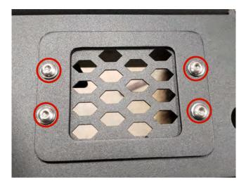
**STEP 6** // If choosing not to use the LED fog lights, install the (2) mesh grille inserts into the bumper using the (4) M6x1.0x15mm screws, lock washers, and nuts.
