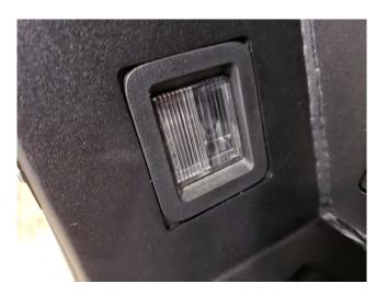
**STEP 4** // Using a trim panel removal tool, push in the plastic tabs around the license plate lights and remove them from the factory bumper. Install these in the new bumper by gently pushing them in place until they click in.
