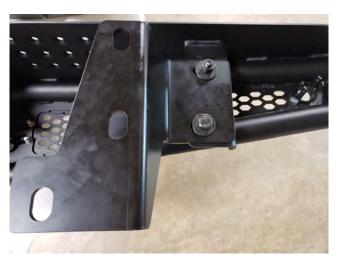
**STEP 8a** // If your vehicle is not equipped with a trailer hitch receiver, install the bumper bracket to the bumper using the (1) bolt plate, (1) M10x1.5x25mm bolt, (2) M10 flat washers, (2) M10 lock washers, and (1) M10 nut. Then remove the factory triple bolt plate and insert through the back of the bumper mount plate.
