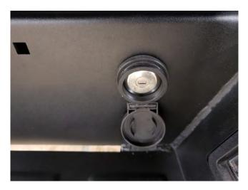
**STEP 3** // Using your factory ignition key, turn the spare tire lock counter clockwise and remove the spare tire lock from the factory bumper. Transfer it to the new bumper.
