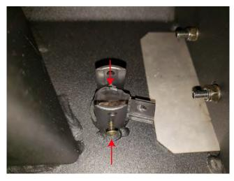
**STEP 5** // If equipped re-install the factory reverse sensors w/ the rubber grommet flush to the outer face of the bumper.
