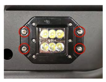
**STEP 7** // **Optional Light:** If choosing the LED fog light option, install the (2) LED Fog lights into the bumper using the (4) M6x1.0x15mm screws, lock washers, and nuts.
