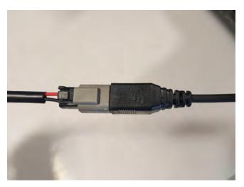
**STEP 10 // Optional Light Wiring:** Connect the (2) LED Fog lights into the supplied harness. Be sure to zip tie the access wiring away from any damage that could occur.
