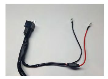
**STEP 11** // **Optional Light Wiring:** Install the Red 12+volt wire to the positive battery terminal. Connect the Black ground wire to the negative battery terminal. Mount the fuse in a safe location away from any damage that could occur. Tuck away any extra wiring.
