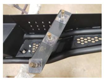
**STEP 8a** // If your vehicle is not equipped with a trailer hitch receiver, remove the factory triple bolt plate and insert through the back of the bumper mount plate.
