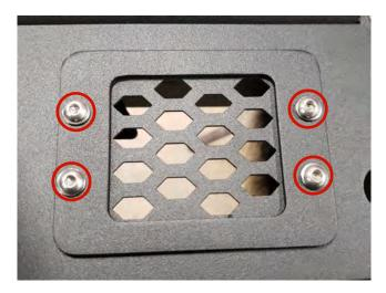
**STEP 6** // If choosing not to use the LED fog lights, install the (2) mesh grille inserts into the bumper using the (4) M6x1.0x15mm screws, lock washers, and nuts.
