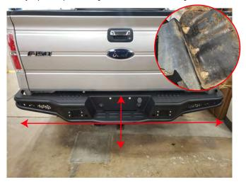
**STEP 9** // Attach the prerunner bumper to the vehicle using the factory (6) 21mm nuts. Be sure to center the bumper, and adjust height of bumper to desired location. Then reinstall the trailer plug and license plate harnesses. If equipped, reinstall the backup camera harnesses.
