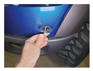
**Step 3** Carefully pull out the fender light from the rubber grommet.
