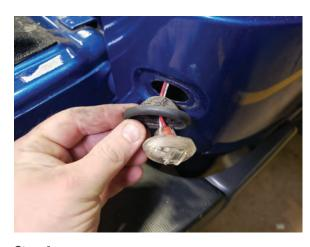
**Step 4**Remove the rubber grommet from the body of the fender, and carefully pull the light and harness from the fender.
