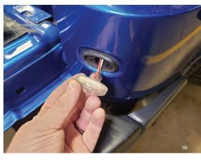
**Step 3**Carefully pull out the fender light from the rubber grommet.
