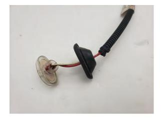
**Step 5**Carefully remove the factory rubber grommet from the factory light and harness. Transfer the rubber grommet to the new light.
