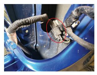
**Step 2**Locate and unplug the factory fender light harness from the main taillight harness.
