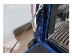
**Step 6\\** Install shock as shown above.
