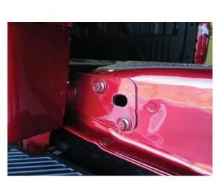
**Step 3\\**Remove the (2) 10mm bolts on the lower tailgate bracket.
