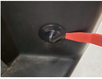
**Step 1\\**Using a flat head screw driver or trim panel removal tool, carefully pry the factory license plate light from the bumper.
