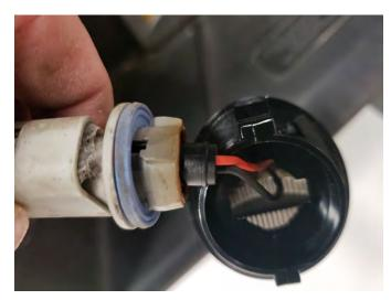
**Step 3\\**Plug the new light harness into the factory light bulb socket. \*\*Note: Test lights for proper function at this point. If the light is not working, unplug the harness from the socket and rotate 180 degrees and test light again.
