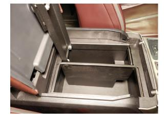
Step 5 Carefully slide the center console vault into the center console. Make sure its seated all the way into the center console.
