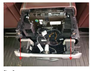
Step 3 Gently pull the rear center console cover away from the center console. Carefully unplug all connections, and remove the cover.
