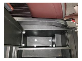
**Step 8**Align the drilled hole locations with the metal bracket plate underneath the console and secure the vault using the (4) M6x1.0x40mm bolts, lock washers, and flat washers.
