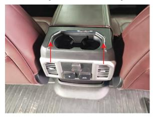
Step 1 Begin by carefully pulling up to release the rear cup holders located on the center console.
