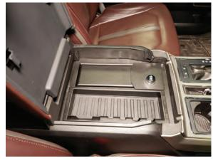
**Step 9**Insert a foam pad to cover the mounting bolts.
