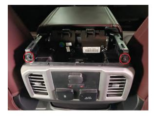
Step 2 Locate, and remove the (2) 7mm screws securing the rear center console cover.
