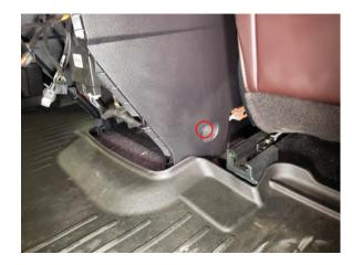
Step 4 Slide both front seats all the way forward to gain access to the (1) 10mm bolt on each side of the lower center console. Remove the bolts.
