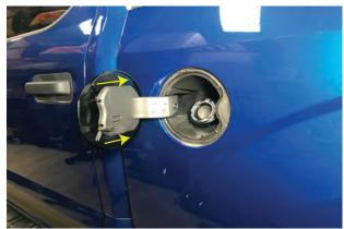
//Step 2: Slide the new fuel door into the fuel door arm tracks opposite as removal. Slide it until it clicks into place.
