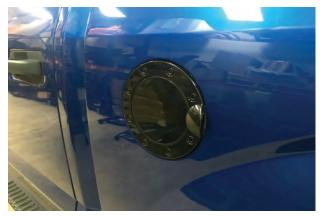
//Step 3: Stick the fuel door cover to the vehicles fuel door. Apply even, firm pressure to the cover. Once fully adhered, installation is now complete.
