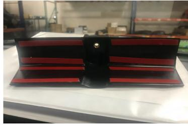
// Step 2: Peel the double sided tape from the mount, and apply firm even pressure to the dash to ensure proper adhesion.
