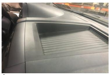
//Step 1: Empty all contents in dash tray to make room for the phone mount. Clean the front of the dash tray with isopropyl alcohol.
