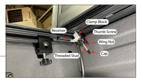
With a helper, place the tonneau cover on the vehicle. The panel with the pre-installed threaded stud with be all the way at the front of the bed. Pull the stud down out of channel. Center the tonneau cover between the bed rails and install the aluminum clamp block. The hook on the clamp block will catch the receiver on the side rail as shown. Use the supplied thumb screw to tighten the clamp block to the side rail. Loosely install the wing nut and rubber cap.
