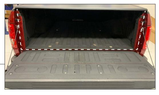
Install the supplied weather stripping around the tail gate to help reduce water intrusion.
