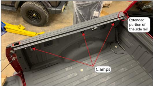
Identify and mount the side rails, the extended portion of the rail will face forward. Using the supplied clamps and Allen bolts, clamp the rails to the bed. While tightening the Allen bolt, use
