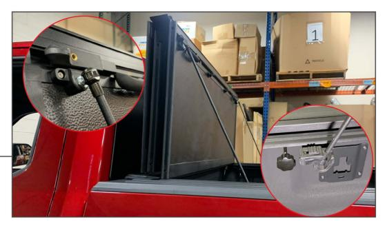
Install the supplied prop-rods. These will hold the tonneau up and out of the way when the bed is in use. Press the prop-rod ball socket onto the tonneau cover ball stud. Clip the other end of the prop-rod into the rail lock. Adjust the rail lock front-to-back so that the tonneau cover is perpendicular to the bed then tighten the thumb screw. When prop-rods are not in use, unclip them from the bed rail and rotate them 90\* and clip them into the tonneau cover for storage.
