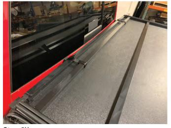
**Step 8\\**Fold the tonneau cover back and secure the cover using the pre-installed straps when not in use.
