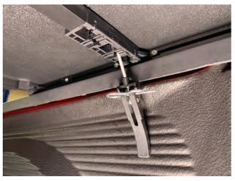
**Step 6\\**Insert the supplied cotter pin to lock the latches in place.
