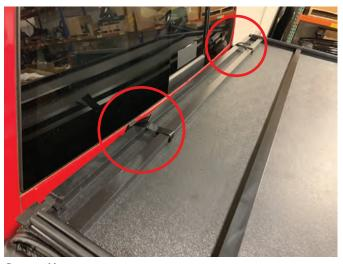
**Step 1\\**Place the tonneau cover on the bed of the vehicle. The shorter latch component will be closest to the cab. The longer strap component will be on top.
