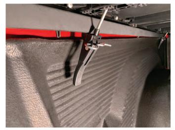
**Step 7\\**Fold down the cover and repeat the process for the rear latches.
