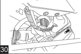
Remove panel below steering column to gain access to trigger wires.
