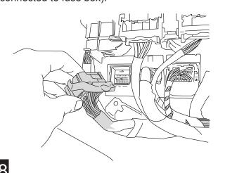
Locate the vehicle's Door Ajar Switch wires on the removed connector as indicated in chart and diagram below according to vehicle model year.
