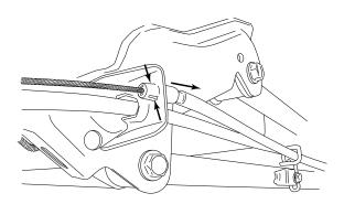
Attach brake cable guide to supplied Brake Cable Bracket (23) and mount bracket with supplied hardware. Reattach brake cable and readjust brake cable adjustment nut to original position.
