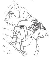
Splice Power Step trigger wires into the Door Ajar wires with provided Posi-Tap™ splicers. The Power Step trigger wires color coordinate with the factory Door Ajar wires. Follow the steps below to correctly splice wires.
