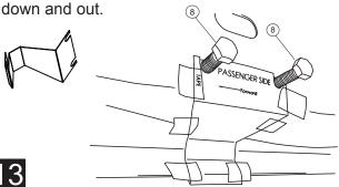
Mark appropriate holes as indicated with a center punch. Front linkage marked "Front" and Rear linkage marked "Rear".
