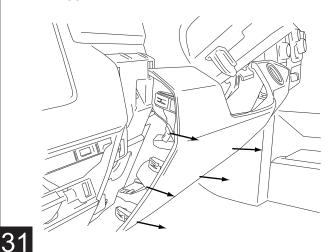
To gain access to white connector panel against driverside firewall panel (inside cab of vehicle), just behind e-brake pedal, some vehicles will have a mounted component that will need to be removed. The component's bracket can be removed by the three fasteners indicated below.
