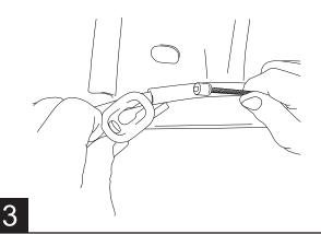
Remove brake cable guide from frame by depressing locking tabs and sliding guide out through hole. Unthread brake cable from frame mount.
