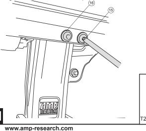
With linkage in position insert Hex bolts into rivet nut locations. Snug bolts but do not tighten. Note: Pre threaded bolt will attach to slot centered on linkage. Idler linkages will use 2 of the 3 mount points
