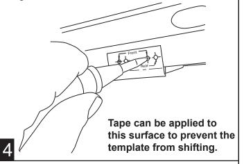
Using a marker draw cross hatch to verify bit does not walk while drilling.
