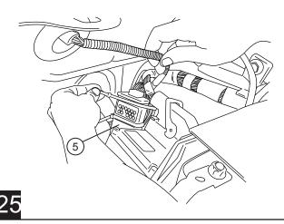
Remove fuse from Power Step Wire Harness.
