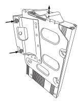
Locate white connector panel against driverside firewall panel, just behind e-brake pedal. Locate three connectors as shown below and connect Powerstep trigger wires as indicated in the chart.
