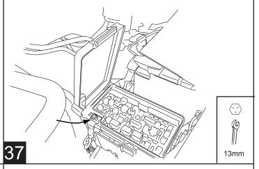
Locate and remove Black Connector with Gray latch on bottom side of fuse box (labeled "G" where connected to fuse box).
