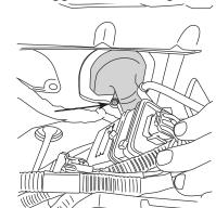
Tape leading end of wires together and push through rubber boot to cabin side of the firewall. Silicon lubricant may be used for ease of passage. The trigger wires will come out just above and to the left of the brake pedal.
