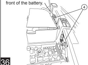
Remove fuse box lid and fuse box power lead with 13mm wrench. While depressing release tabs, lift fuse box to view bottom side.
