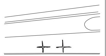
Pre drill hole using an 1/8" drill bit. Next drill holes to 9/32". Debur all surfaces. NOTE: Filing of hole may be required if drill bit wandered. After drilling apply paint to prevent rusting.
