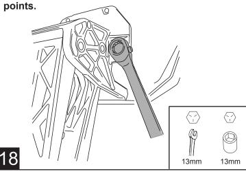
Using a 13mm wrench tighten two hex bolts on linkage. Torque to 16 ft-lbs.
