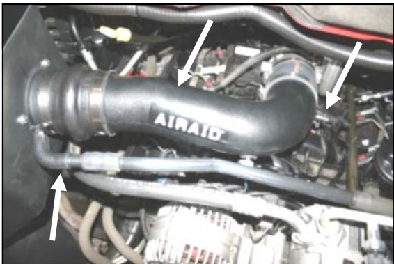
12. Install the Airaid intake tube into the hump hose first, and then into the reducing coupler. Adjust for fit, and then tighten all four hose clamps. 2004-08 Models: Reconnect the breather by sliding the 3/4" x 2" hose (#24) over the factory breather tube. Next insert the 1/2" to 3/4" barbed connector (#20) into the 3/4" hose. Now connect the 1/2" rubber elbow (#15) between the 1/2" barbed fitting on the CAD and the previous fitting. Now slide the rubber cap (#14) over the nipple on the Airaid intake tube and secure it with the #14 speed clamp (#16).
