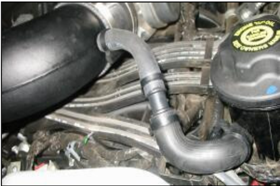
13. 2003 Models: Reconnect the factory breather hose using the 1/2" x 5/8" connector (#21) and 1/2" x 4 1/2" breather hose. Secure the ends with the #16 speed clamps (#17), and the #22 speed clamps (#18) as shown.
