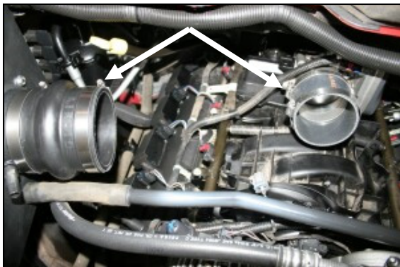
10. Install the supplied reducing coupler (#4), onto the throttle body using one #52 hose clamp (#10) on the throttlebody and one #56 hose clamp (#11) on the open end. Install the hump hose (#5) with two #60 hose clamps (#12) onto the CAD .
