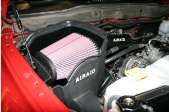
14. Install the Airaid Premium Filter (#1) onto the tube on the filter adapter and tighten the clamp. Next install the weather strip (#7) on the top of the Quick Fit Panel as shown. ( Hint: Start at one end of the CAD and work your way towards the other end. )
