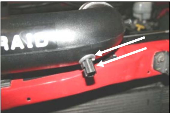
11. Install the supplied grommet (#13) into the Airaid intake tube(#2). Next, carefully install the factory air intake temperature sensor into the grommet in the tube. Make sure it is fully seated into the grommet.
