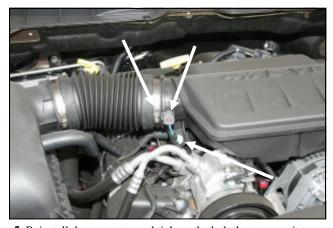
5. Reinstall the resonator and tighten the bolt that secures it to the intake manifold. Reinstall the intake tube, tighten the hose clamp, and reconnect the intake temperature sensor.
