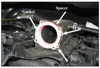
**3.** Install the Poweraid Spacer into the intake manifold as shown. Make sure the spacer is seated correctly over the two alignment pins on the intake manifold. \*Note: Poweraid spacer must be installed with bore protruding into intake manifold away from throttle body. Incorrect installation will hinder performance.
