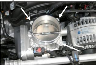
2. Remove the four bolts that secure the throttlebody to the intake manifold. Without disconnecting the wiring harness, remove the throttlebody from the intake manifold and set it aside.
