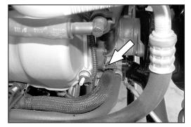
20. On 2002-2007 model year vehicles, use a 8mm socket, remove the stud that retains the oil fill bracket.
