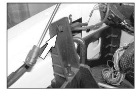
18. Remove the 8mm bolt that retains the air box mount.
