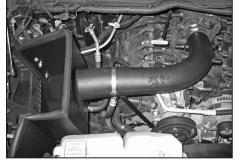
28. Install the K&N<sup>®</sup> intake tube into the silicone hose at the throttle body and align to the mounting bracket, secure the intake tube with the hose clamps provided.
