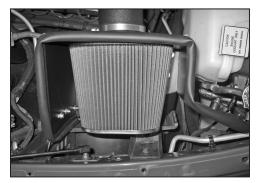
34. Install the K&N $^{\mbox{\tiny B}}$  air filter onto the intake tube as shown.
