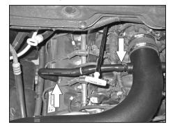
33. On 2008 and later model year vehicles, connect the crank case vent hose assembly to the valve cover port and intake tube vent fitting as shown.
