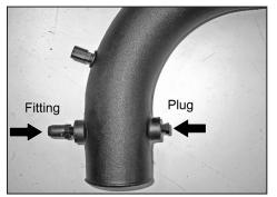
27a. On 2002-2007 model year vehicles, install the NPT fitting and NPT plug as shown. **NOTE: Plastic NPT fittings are easy to cross thread. Install the vent fitting "hand" tight, then turn it two complete turns with a wrench.**
