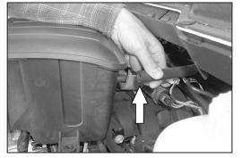
7. On 2002-2007 model year vehicles, disconnect the crank case vent hose from resonator box as shown. Then remove resonator box from vehicle. **NOTE: K&N Engineering, Inc., recommends that customers do not discard factory air intake.**
