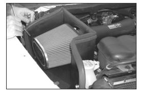
35. Align the heat shield for best clearance then tighten all the brackets.
