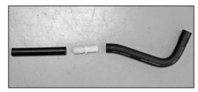
30g. On 2008 and later model year vehicles, insert the provided hose mender into the remaining piece of the factor vent hose and then cut the provided vent hose to 5" length connect onto the hose mender.
