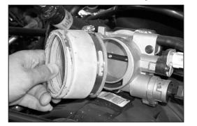
8. On 2002-2007 model year vehicles, loosen hose clamp that retains the rubber hose to the throttle body then remove as shown.
