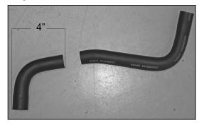
30f. On 2008 and later model year vehicles, cut the factory crank case vent hose 4" from the end as shown.
