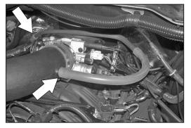
32. On models with the crank case vent tube connected to the passenger side valve cover, connect the provided silicone hose onto the factory vent tube and then route the crank case tube assembly behind the throttle body as shown and connect the open end onto the K&N<sup>®</sup> intake tube.
