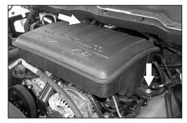
5. Remove the two 10mm bolts that retain the resonator box onto the engine. NOTE: On 2008 and later model year vehicles there will be only one bolt to secure the resonator.
