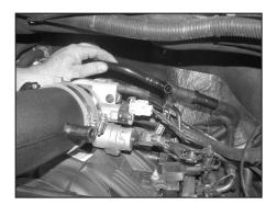
30e. Reinstall the vent tube assembly into the rubber fittings in each valve cover so that the "T" fitting is now on the drivers side of the engine facing forward.
