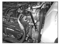
21b. On 2008 and later model year vehicles, install the tube mounting bracket using the bolt removed in the previous step and the spacer provided.
