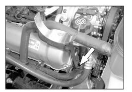
21. On 2002-2007 model year vehicles, install the saddle bracket assembly with the stud that was removed in step 20.
