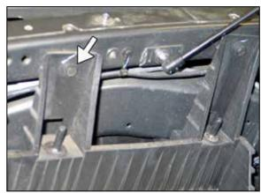
17. Remove the front air box mounting bracket bolt shown.
