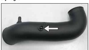
24. Install the inlet air temperature sensor into the grommet installed into the K&N® intake tube as shown.
