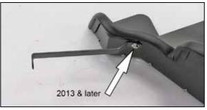
16. Install the heat shield mounting bracket (083103-1) onto the heat shield using the provided hardware.
