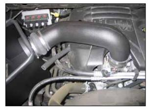
25. Install the K&N® intake tube into the silicone hump hose and then into the silicone hose at the throttle body. Align the heat shield assembly for proper fit and then tighten the heat shield mounting bolts. Also secure the hose clamps securing the intake tube.
