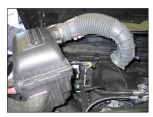
5. Disconnect the factory intake hose from the throttle body, then lift up the air box assembly and remove from the vehicle.
