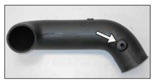
22. Install the 1/4 NPT vent fitting into the K&N® intake tube as shown.
