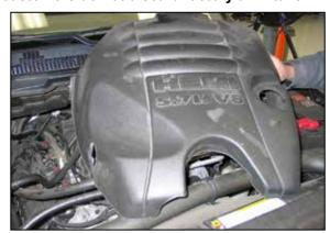
6. Lift up the engine cover to dislodge it from the mounting posts and then remove it from the vehicle.
