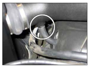
26. Connect the crank case vent hose to the fitting installed into the K&N® intake tube and secure with the provided hose clamp.
