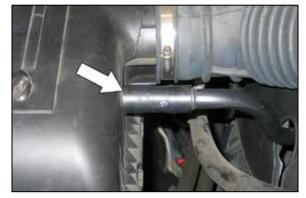
4. Disconnect the crank case vent hose from the air box.
