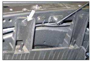
17. Remove the front air box mounting bracket bolt shown.
