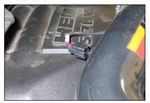
27. Connect the provided inlet temperature sensor extension into the factory wiring harness and then connect the other end to the inlet temperature sensor.
