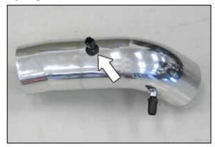
24. Install the inlet air temperature sensor into the grommet installed into the K&N $^{\circ}$  intake tube as shown.
