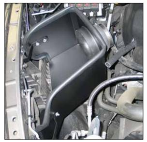
11. Reinstall the engine cover onto the mounting studs and route the crank case vent hose through the opening.
