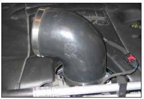
20. Install the provided silicone hose (084086) onto the throttle body and secure with the provided hose clamp.
