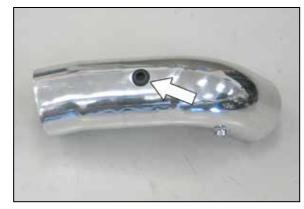
21. Install the provided grommet into the K&N $^{\mbox{\scriptsize \$}}$  intake tube as shown.
