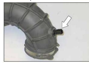
23. Remove the inlet air temperature sensor from the stock intake tube.
