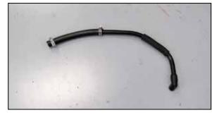
9. Install the provided vent hose onto the cut hose with the provided hose clamps as shown.
