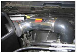
25. Install the K&N<sup>®</sup> intake tube into the silicone hump hose and then into the silicone hose attached to the throttle body. Align the heat shield assembly for proper fitment. Tighten the heat shield mounting bolts and hose clamps securing the intake tube.
