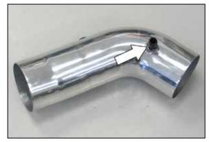
22. Install the 1/4 npt vent fitting into the K&N<sup>®</sup> intake tube as shown.
