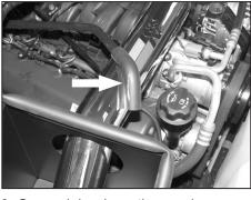
39. On models where the crank case vent hose is connected to the passenger side valve cover, remove the factory 90° coupling hose from the plastic vent tube.
