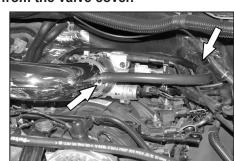
40. On models with the crank case vent tube connected to the passenger side valve cover, connect the provided silicone hose to the factory vent tube. Then, route the crank case vent tube assembly behind the throttle body as shown. Connect the open end onto the K&N® intake tube.
