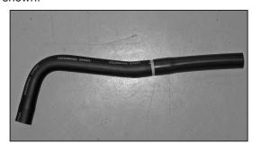
41c. On 2008 and later model year vehicles, install the provided hose mender and crank case vent hose onto the cut factory vent hose as shown.
