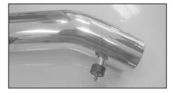
26. Install the rubber mounted stud into the threaded boss on the K&N® intake tube as shown.
