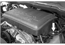
5. Remove the two 10mm bolts that retain the resonator box onto the engine.
