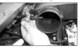
4. On models that come equipped with air temp sensors, unplug the air temp. sensor electrical connection as shown.
