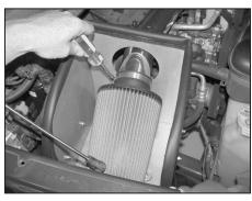
42. Install the air filter and secure with the provided hose clamp as shown.
