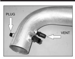
25b. On 2008 and later model year vehicles, install the ½"npt vent fitting and plug as shown.
