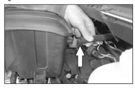
7. On 2002-2007 model year vehicles, disconnect the crank case vent hose from resonator as shown, then remove resonator from vehicle.
