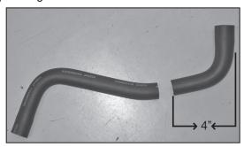
41b. On 2008 and later model year vehicles, cut the factory crank case vent hose 4" from the end as shown.
