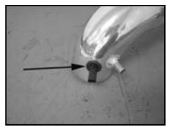
Step 12 Install the grommet into the tube. Reinstall the factory IAT sensor.
