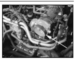
Step 6 Install the throttle body adapter ring onto the throttle body.
