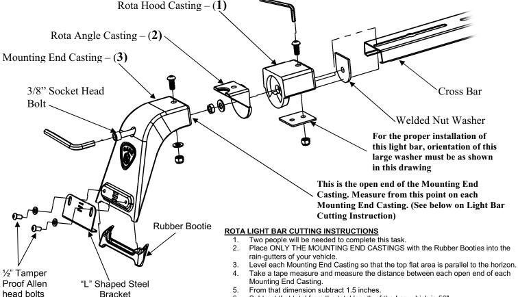
MATERIALS NEEDED: Hammer, center punch, pencil MATERIALS FURNISHED: One hardware pack, two end castings, four Rota castings, cross bar, instruction page.
