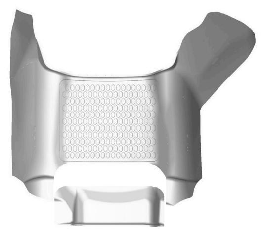
IF YOUR DODGE RAM TRUCK HAS THE STORAGE COMPARTMENT LOCATED ON THE TRANSMISSION TUNNEL IN FRONT OF THE CENTER SEAT, YOU WILL NEED TO TRIM YOUR CENTER HUMP LINER AS SHOWN ABOVE. TO TRIM, USE A PAIR OF HEAVY SHEARS OR A UTILITY KNIFE AND USE THE OFFSET IN THE LINER AS YOUR TRIMMING GUIDE.
