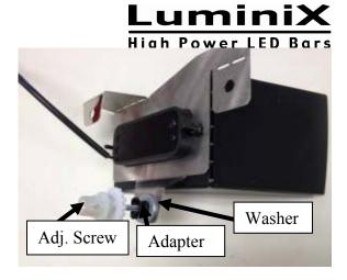
Place plastic adapter through 17/32" washer and into square hole on Putco fog lamp assembly as shown above. Thread adjustment screw into plastic adapter. (shown above)
