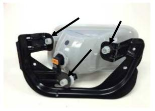
When factory fog lamp assembly is removed, use pliers to unclip (3) plastic clips (locations shown above) to remove bracket from factory fog lamp. Driver side is shown
