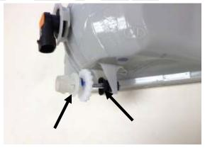
Remove adjustment screw and plastic adapter from factory fog lamp.(will be used in Step 5) Place fog lamp aside, this will not be used.
