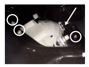
Remove (3) 10mm Bolts from factory fog lamp bracket. Unplug bulb from factory fog lamp and remove Lamp assembly from truck. Passenger side is shown. Repeat on Driver side. (wire loom clips my need to be removed to get fog lamp out)
