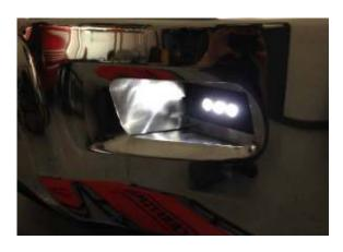
Mount light assembly into truck in reverse order of Step 2 using (3) factory 10mm bolts. Repeat Steps 3-6 on passenger side.
