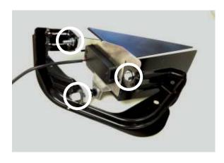
Snap adjustment screw clip back into factory bracket (removed in Step 3). Secure upper mounting locations with the 5/16" hardware. (Do not install washer on same side as lock nut) Use 1/2" wrench to tighten hardware.
