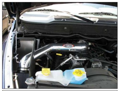
AEM® intake system installed
