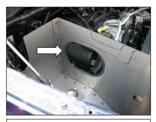
I. Attach the rubber edge trim to the heat shield opening.
