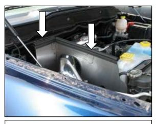
q. Attach the sponge gasket to the top of the heat shield.
