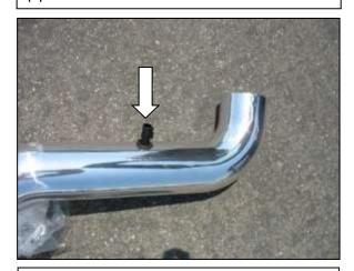
k. Insert the IAT sensor into the inlet pipe.
