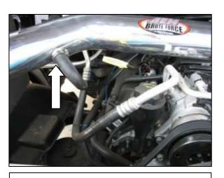
n. Attach the breather hose to the inlet pipe as shown. Secure with the provided hose clamp. Make sure that the rubber elbow is not kinked for air flow.
