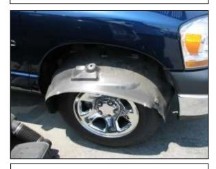
h. Remove the fender liner on the passenger side to access the air box mount.
