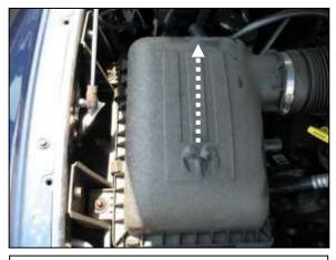
g. Pull the air box straight up along with the inlet tube. Remove the intake plenum and the coupler attached to the throttle body.
