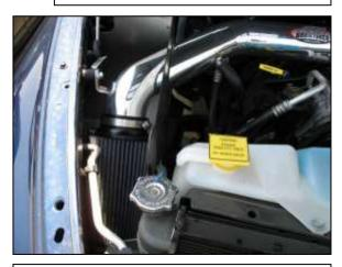
o. Attach the air filter as shown. Secure with #60 hose clamp. Check for clearance around the heat shield and A/C lines.
