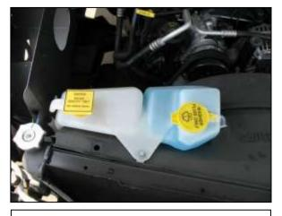
g. Reinstall the washer/coolant overflow reservoir.
